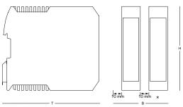
H= 99mm,\* Version without or with power module: B= 22,5mm(+ 10mm ventilation on both sides) or 45mm(+ 10mm ventilation on both sides),T=116mm
