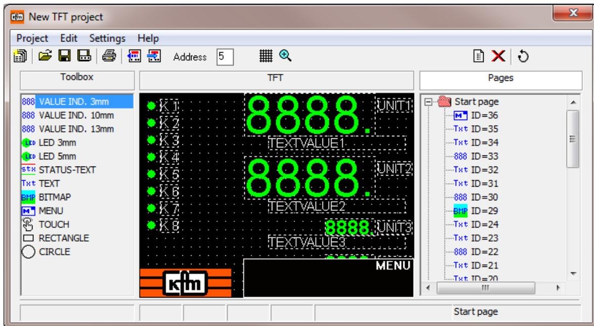
TFT- displays from KFM- series 803 and 903 can be changed or completely new designed with this program.
